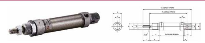
Working Temperature: 0°C (-20°C with Dry Air) - Max +80°C, Working Pressure: 1 - 10bar, Fluid: Filtered Compressed Air, Either Lubricated or Non-Lubricated, Materials: Heads: Anodised Aluminium, Bush: Self Lubricating Sintered Bronze, Piston: Brass, Barrel: AISI304 With Rolled Front And Rear Heads, Piston Rod: Rolled AISI 304, Seals: Special Nitrile Pre-Lubricated For Minimum Friction, Long Life And Non Lube Service, Standard Cushioning Rings On All Sizes.
