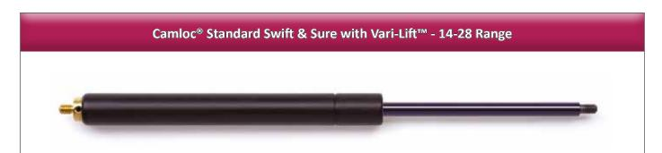
Features: Type: Variable Force, Rod Diameter: 14mm, Tube Diameter: 28mm, Thread M10 x 1.5, Force Range: 200 - 2500N, Material: Nitrided steel piston rod - black powder coated steel tube - nylon/steel end connectors, Swift & Sure - Vari-Lift gas springs come gassed to maximum pressure. Boxed as a pair and fitted with BEA-B6 end fittings - instructions and an allen key for adjusting force in-situ. Please note: Extended lengths quoted are between centres of BEA-B6 end fittings.
