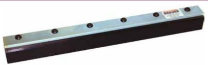
Technical Details: Material: Aluminium/Zinc plated steel, Weight: 1.35Kg, Standard Gap: 0.5-0.10mm, DBA at: 5.5 bar is 80, Standard Inlet Threads: 1/4" BSP
