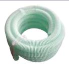
Clear PVC Reinforced With Blue Tensile Steel Wire Spiral - Suitable For The Suction And Discharge Of Water, Slurry, Some Chemicals, Sewage, Granules And Other Waste Materials - Particularly Suitable For Horticultural And Marine Industries - Resistant To Reducing Agents And Diluted Acids - Vacuum: 570mm Hg = 75% at 20°C Temperature Range: -15°C to +65°C - Cold Bend: -45°C - Additional carriage charges apply to: LDH50/30
