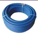
Resistant To A Wide Range Of Chemicals - High Resistance To Acids And Alkalis - Silicone Free - Abrasion Resistant - Made From Cadmium Free Materials - Low Toxicity - Suitable For Food Use - 3:1 Safety Factor @20°C - Temperature Range: -15°C to +60°C - Note: Standard Colour is Blue. Other colours are available subject to Minimum Order Quantity
