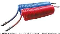
Fitted With BSPT Press-in Swivel Couplings - Complete With Springs - Excellent Flexibility - High Resistance To Oil, Petrol, Organic And In-Organic Media - Light Weight - Expansion And Retention For Ease Of Use - Temperature Range: -40°C to +80°C - Maximum Working Pressure: 15bar
