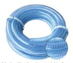
Clear PVC Reinforced With Blue Tensile Steel Wire Spiral - Suitable For The Suction And Discharge Of Water, Slurry, Chemicals, Sewage, Granules And Other Waste Materials - Can Also Be Used For Suction And Discharge Of Foodstuffs - Vacuum: 711mm Hg = 94% at 20°C - Temperature Range: -15°C to +65°C - Cold Bend: -45°C
