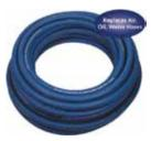
Specification - Exterior: Blue Colour - Working pressure: 20Bar - Bursting Pressure: 60 Bar - Tube Compound: SBR / NBR - Cover Compound: NBR / EPDM - Temperature: -20°c to +90°c
